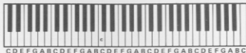
"Normal" CS-80 keyboard range (Feet Selector at 8'). Middle "C" equals 8' pipe on organ.
